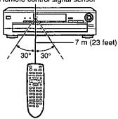
Aim at the sensor, avoiding obstacles, at a maximum range of 7 m (23 feet) directly in front of the unit
